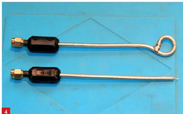
Fig. 1: TinySA-Ultra displaying noise from a Wall Wart PSU. Fig. 2: Completed E-Field probe (top), H-Field probe (bottom). Fig. 3: Cable and clip-on ferrites. Fig. 4: Completed probes before applying insulation. Fig. 5: Close up view of loop before soldering. Fig. 6: Close in view of the H-Field loop. Fig. 7: TinySA-Ultra measuring noise from the sockets of a Racal RA6790GM Serial Interface.
